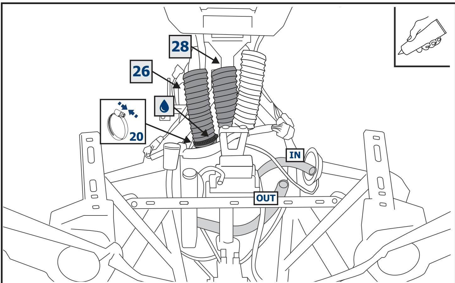
**EN** Install protective thermal hose ( $l = 0.1 \text{ m}$ ) on air ducts in such a way that the quad-bike steering column could not wear down them.
